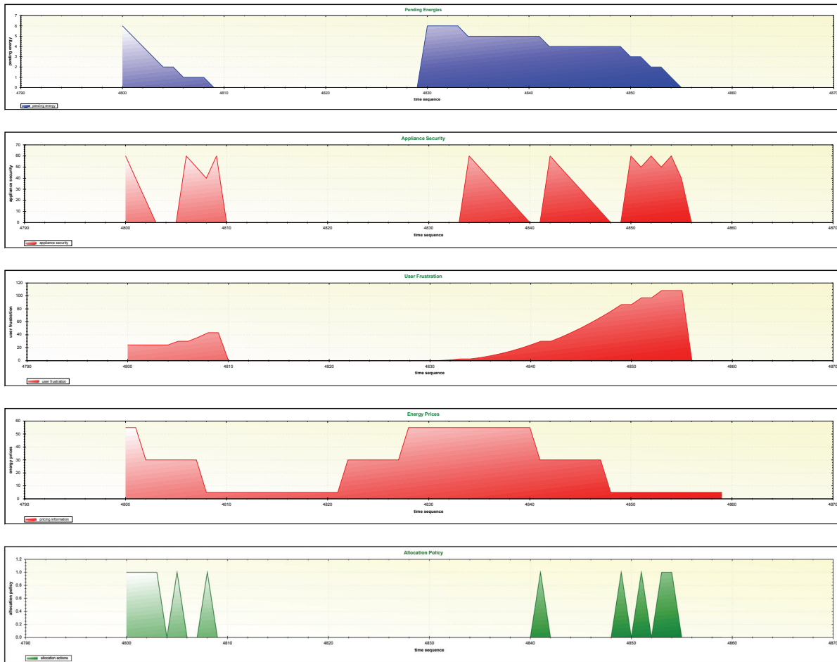
Figure 10: Sample results for S2A. From top to bottom: pending energy, appliance security penalty, usability penalty, smart pricing, and energy allocation actions.
