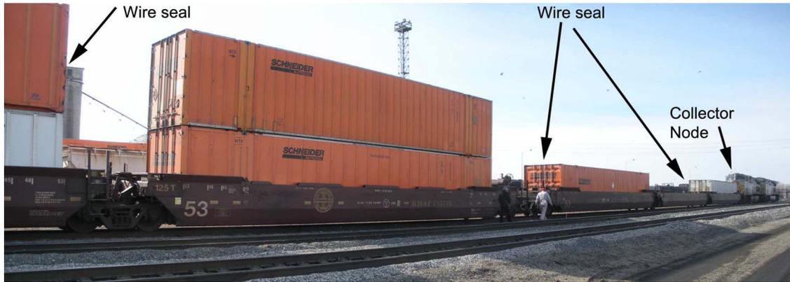
Fig. 8. Collector node and sensor deployment during short-haul rail trial.
